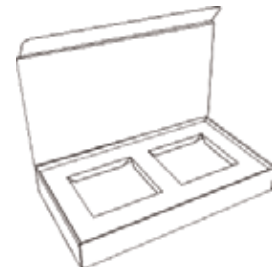
M0073 13" x 7" x 1-3/4" 2 Side Rollover w. Front Tuck Super Panel on Inside Lid Custom Insert
