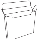
4308 11 3/4" W x 10" H 2" Fixed Capacity Side "Wings" and Fold Over Tuck Flap 1-2-3 Bottom
