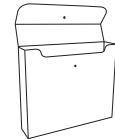
42010 11 3/4" W x 10" H 2-1/2" Fixed Capacity Fold Over Flap Auto Lock Bottom *Various Capacities Available
