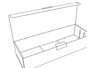
M0079 20-1/16" x 7-3/8" x 4" 2 Side Rollover w/Front Tuck & Locking Tab Custom Insert (not shown)
